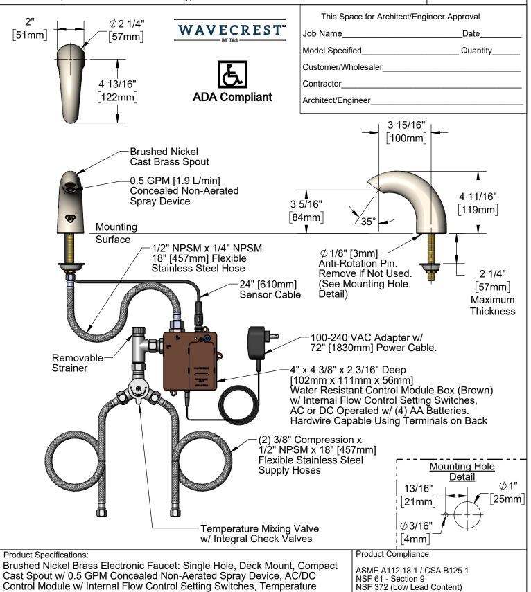
Control Module w/ Internal Flow Control Setting Switches, Temperature Control Mixing Valve w/ Integral Check Valves & 18" Hot & Cold Supply
