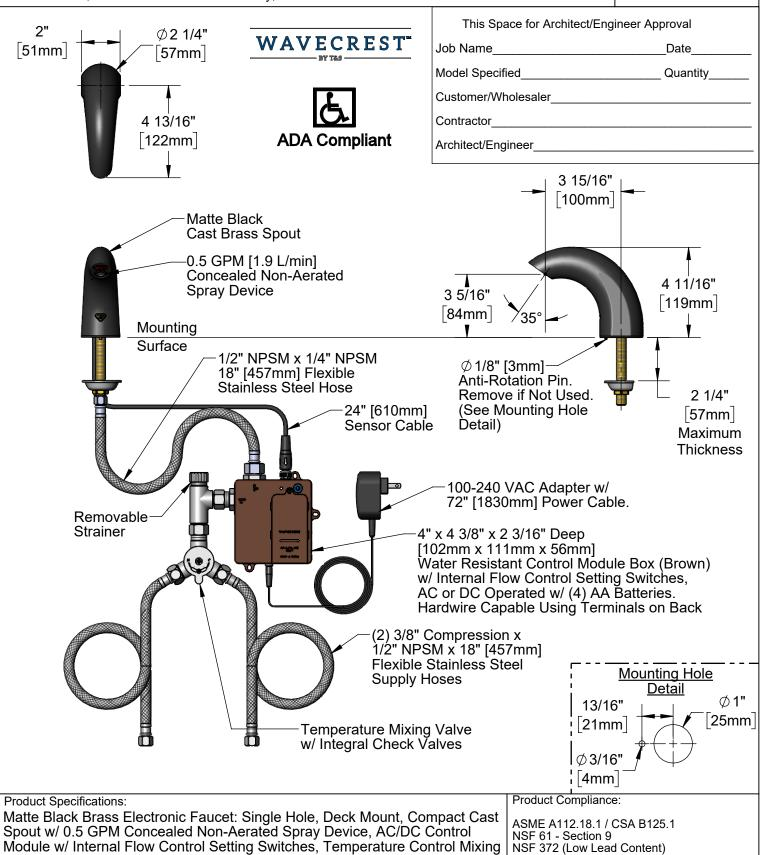
Module w/ Internal Flow Control Setting Switches, Temperature Control Mixing
