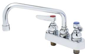
B-1110 4" centers with 6" Swing Nozzle B-1110-XS With 2" extended shanks
