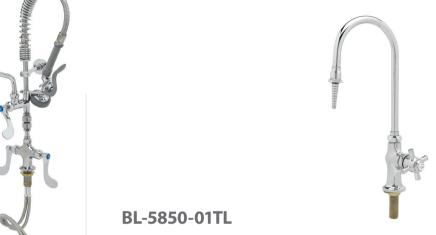
Single hole single temperature tin-lined deck mount faucet with polished chrome plated brass body, 5 7/8" swivel/rigid gooseneck with serrated tip outlet, fast self-closing cartridge, 4-arm handle and 1/2" NPSM male inlet. Certified to ASME A112.18.1/CSA B125.1 and NSF 372.
