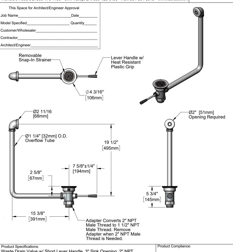
Waste Drain Valve w/ Short Lever Handle, 3" Sink Opening, 2" NPT Male Outlet, 1 1/2" NPT Male Adapter & Overflow Tube w/ Head Asm
