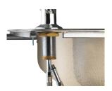
Step 1: Insert flex line inlets and tighten by hand. Apply plumber's putty to underside of body and insert into mounting hole. With wrench, tighten the locking nut.
