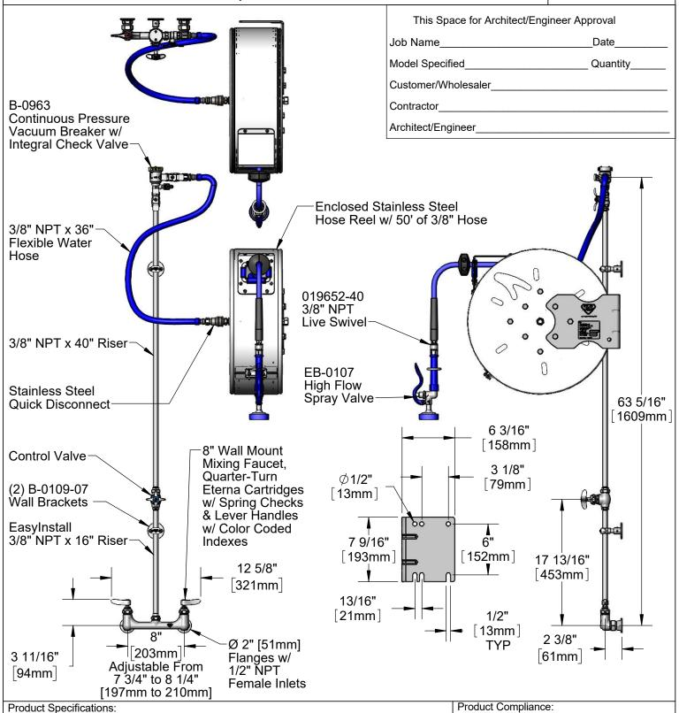
Enclosed Stainless Steel Hose Reel w/ 50' of 3/8" Hose, High Flow Spray Valve w/ Swivel, Vacuum Breaker, 3/8" NPT Flexible Connector, 8" Wall Mount Mixing Faucet & Control Valve
