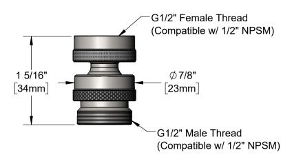
DISCLAIMER: This non-pressurized DuraPull swivel assembly is not designed or rated for the standard typical T&S or Equip PRUs with pressurized flexible hoses.
