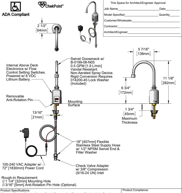
Chrome Plated Brass Above Deck Electronics Faucet, Single Hole Single Temperature Deck Mount, Swivel/Rigid Gooseneck, 0.5 GPM VR Non-Aerated Spray Device, Battery or AC Adapter Powered, Flexible Stainless Steel Supply Line & 3/8" Compression Inlet
