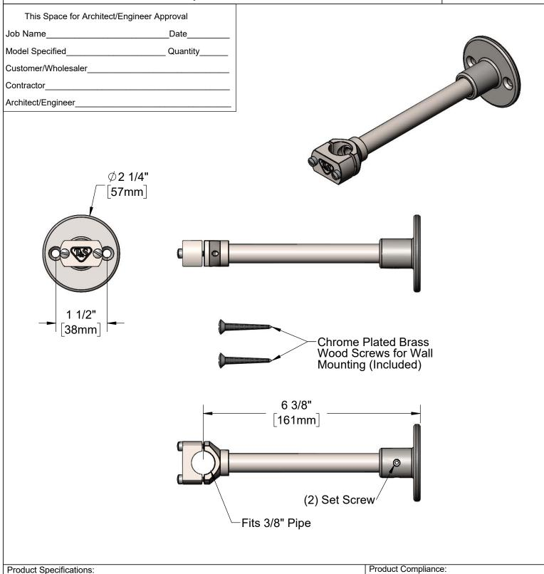
6" Wall Bracket Assembly for 3/8" Pipe w/ Mounting Hardware
