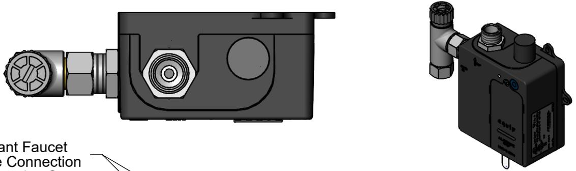
Water Resistant Faucet Sensor Cable Connection (Remove Protective Cap to Connect Cable)
