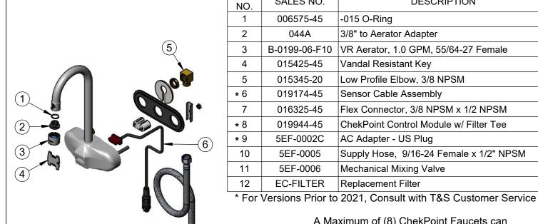
ITEM SALES NO. **DESCRIPTION** -015 O-Ring 3/8" to Aerator Adapter VR Aerator, 1.0 GPM, 55/64-27 Female Vandal Resistant Key Low Profile Elbow, 3/8 NPSM Sensor Cable Assembly Flex Connector, 3/8 NPSM x 1/2 NPSM ChekPoint Control Module w/ Filter Tee AC Adapter - US Plug Supply Hose, 9/16-24 Female x 1/2" NPSM Mechanical Mixing Valve Replacement Filter
