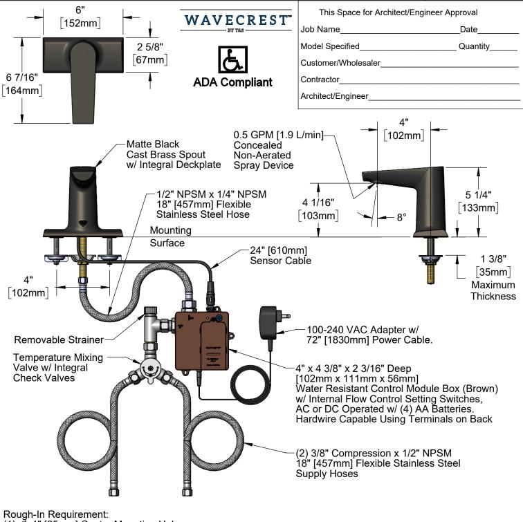
(1)  $\bigcirc$  1" [25mm] Center Mounting Hole (2)  $\bigcirc$  1 1/8" [28mm] Mounting Stud Holes (on 4" Centers)
