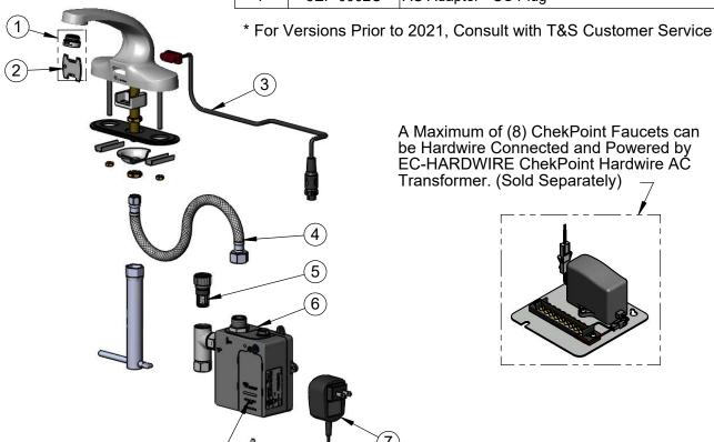
A Maximum of (8) ChekPoint Faucets can be Hardwire Connected and Powered by EC-HARDWIRE ChekPoint Hardwire AČ Transformer. (Sold Separately)
