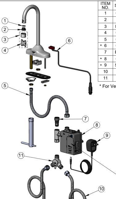
SALES NO. **DESCRIPTION** 006575-45 -015 O-Ring 044A 3/8" to Aerator Adapter B-0199-06 Aerator, Vandal Resistant 015425-45 Vandal Resistant Key 016297-45 Inlet Hose, Faucet, 1/2" NPSM-F x 1/4" NPSM-F 019174-45 Sensor Cable Assembly EC-FILTER Replacement Filter ChekPoint Control Module w/ Filter Tee 019944-45 5EF-0002C AC Adapter - US Plug 5EF-0005 Supply Hose, 9/16-24 Female x 1/2" NPSM 5EF-0006 Temperature Mixing Valve
