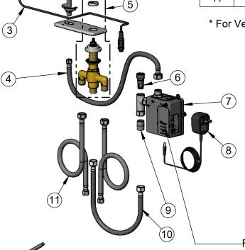
A Maximum of (8) ChekPoint Faucets can be Hardwire Connected and Powered by EC-HARDWIRE ChekPoint Hardwire AĆ Transformer. (Sold Separately)
