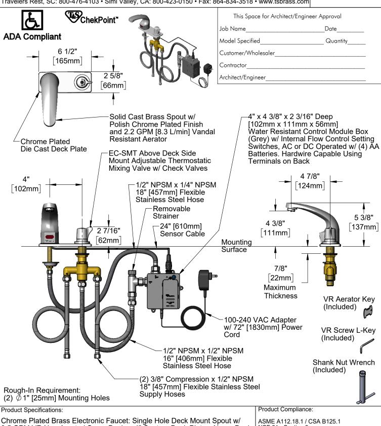
Chrome Plated Brass Electronic Faucet: Single Hole Deck Mount Spout w/ 0.5 GPM VR Non-Aerated Spray Device, 4" Centers Deck Plate, Above Deck Side Mount Adjustable Thermostatic Mixing Valve w/ Check Valves, AC/DC Control Module with Internal Flow Control Setting Switches, 18" Hot & Cold Supply Stop Flexible Connector Hoses
