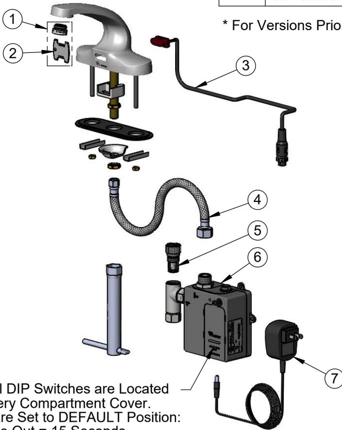
A Maximum of (8) ChekPoint Faucets can be Hardwire Connected and Powered by EC-HARDWIRE ChekPoint Hardwire AC Transformer. (Sold Separately)
