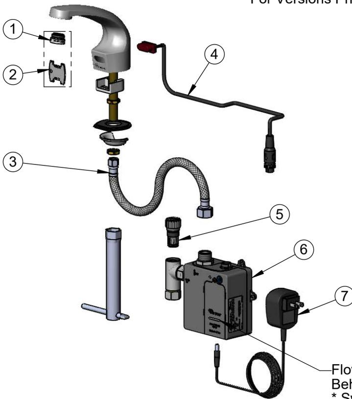
A Maximum of (8) ChekPoint Faucets can be Hardwire Connected and Powered by EC-HARDWIRE ChekPoint Hardwire AC Transformer. (Sold Separately)
