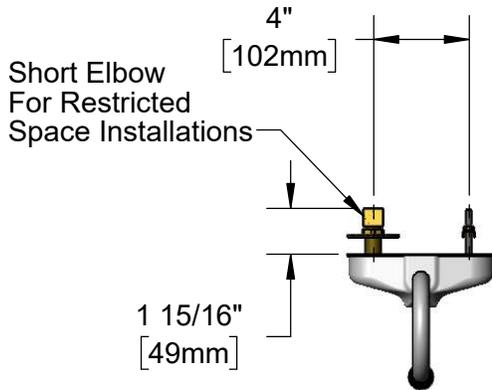
Rigid Gooseneck w/ 0.5 GPM [1.9 L/min] Vandal Resistant Non-Aerated Spray Device
