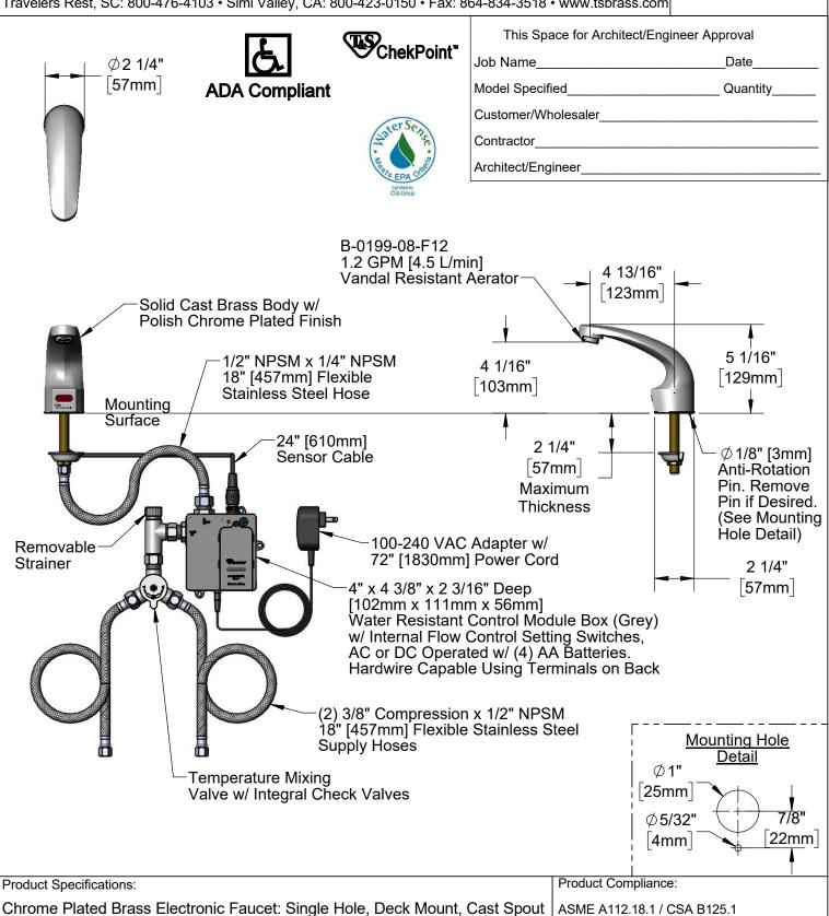
w/ 1.2 GPM VR Aerator, AC/DC Control Module w/ Internal Flow Control Setting Switches, Temperature Control Mixing Valve w/ Integral Check Valves
