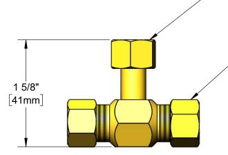
3/8 Compression Fittings w/ Ferrules and Lock Nuts. Remove Lock Nuts and Ferrules for 9/16-24 UNEF Male Thread Connection. (2 Places)
