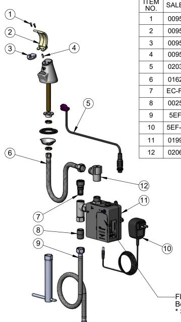
**ITEM** SALES NO. **DESCRIPTION** 009598-45 Mouth Guard Screw (2) 009595-45 Rubber Mouth Guard 009596-40 Mouth Guard Holder 009594-45 Flow Straightener 020315-45 Sensor Cable Assembly - Curved Lens 016297-45 Inlet Hose, Faucet, 1/2" NPSM-F x 1/4" NPSM-F **EC-FILTER** Replacement Filter 002534-25 Close Nipple, 1/2" NPT 5EF-0005 Supply Hose, 9/16-24 Female x 1/2" NPSM 5EF-0002C AC Adapter - US Plug 019944-45 ChekPoint Control Module w/ Filter Tee 020672-40 Flow Control Valve
