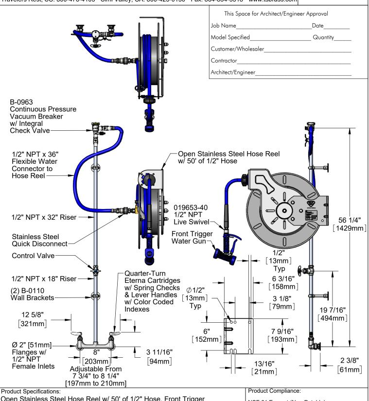
Open Stainless Steel Hose Reel w/ 50' of 1/2" Hose, Front Trigger Water Gun w/ Swivel, 1/2" NPT Vacuum Breaker, 1/2" NPT Flexible Water Connector, 8" Wall Mount Mixing Faucet & Control Valve
