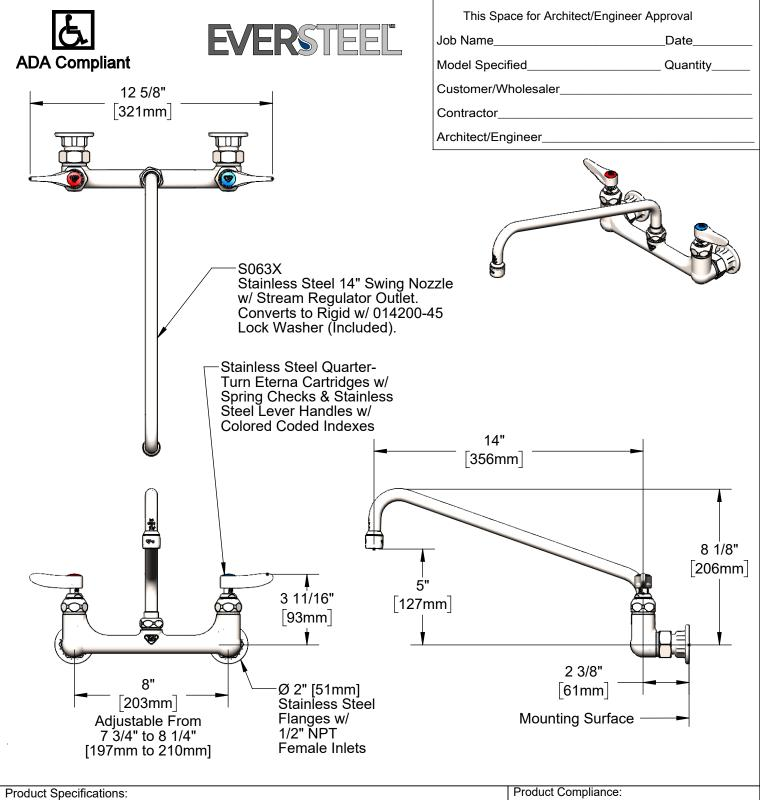
8" Stainless Steel Wall Mount Mixing Faucet w/ SS Quarter-Turn Eterna Cartridges w/ Spring Checks, SS Lever Handles, SS 14" Swing Nozzle & SS 1/2" NPT Female Inlets
