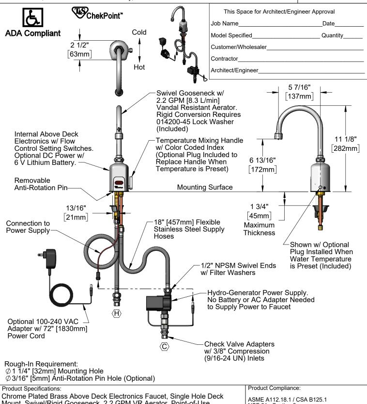
Chrome Plated Brass Above Deck Electronics Faucet, Single Hole Deck Mount, Swivel/Rigid Gooseneck, 2.2 GPM VR Aerator, Point-of-Use Temperature Control, Hydro-Generator Powered, Stainless Steel Flexible Supply Hoses & 3/8" Compression Inlets
