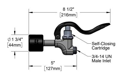
Flow Rate: 1.20 GPM (4.54 L/min) @ 60 psi Spray Force: 7.7 Ozf (218 Gramf) @ 60 psi
