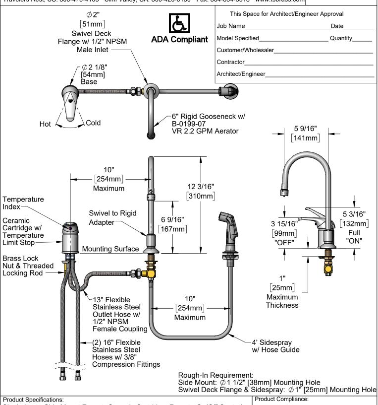
Single Lever Side Mount Faucet, Ceramic Cartridge, Remote On/Off Control Base, Rigid Gooseneck, Vandal Resistant 2.2 GPM Aerator, 4' Sidespray & (2) 16" Flexible Stainless Steel Supply Hoses
