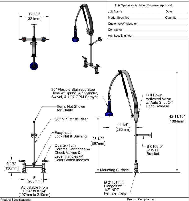
EasyInstall Pull-Down Pre-Rinse Unit: 8" Deck Mount Mixing Faucet, Quarter-Turn Cerama Cartridges w/ Check Valves, Lever Handles, 30" Flexible Stainless Steel Hose, 1.07 GPM Sprayer w/ Ball-Joint Swivel, 6" Wall Bracket & 1/2" NPT Female Inlets with Ø 2" Adjustable Flanges
