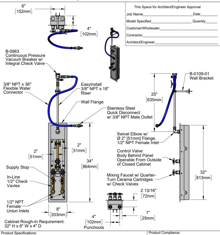
EasyInstall Hose Reel Recess Mounted Cabinet, Concealed Bypass Mixing Valve, Cerama Cartridges w/ Check Valves, Supply Stops, 1/2" NPT Female Union Inlets, Control Valve w/ Cerama Cartridge, 1/2" NPT Riser, Check Valves, Swivel Elbows w/ 1/2" NPT Female Inlet, EasyInstall 3/8" NPT x 18" Riser, 6" Wall Bracket, Continuous Pressure Vac. Breaker w/ Integral Check Valve, Removable Wall Flange,
