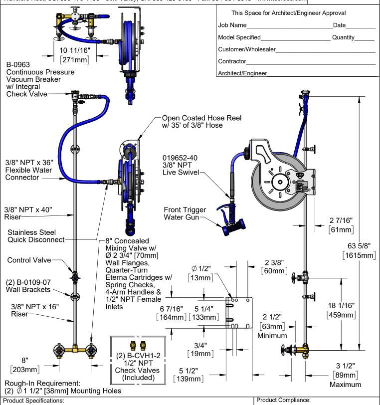
Open Coated Hose Reel w/ 35' of 3/8" Hose, Blue Front Trigger Water Gun w/ Swivel, Vacuum Breaker, 3/8" NPT Flexible Water Connector, 8" Concealed Wall Mount Mixing Faucet, Control Valve & (2) Check Valves
