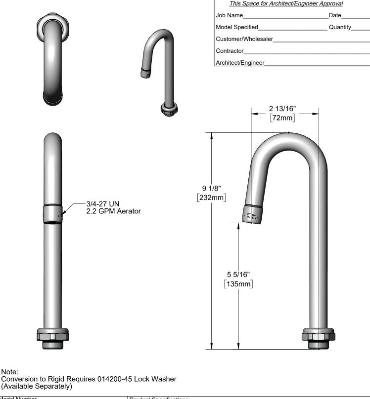
Model Number **Product Specifications:** 5SP-03A 3" Swivel Gooseneck w/ 2.2 GPM Aerator **Product Compliance:** ASME A112.18.1 / CSA B125.1 NSF 61 - Section 9 NSF 372 (Low Lead Content) 2 Saddleback Cove, P.O. Box 1088 Travelers Rest, South Carolina 29690 Phone: 800.891.4808 Fax: 800.868.0084 equip Foodservice Accessories equip.tsbrass.com TRK JRM Drawn: Checked: Approved: JHB Date: 10/30/23 Scale: 1:2 Sheet: 1 of 1
