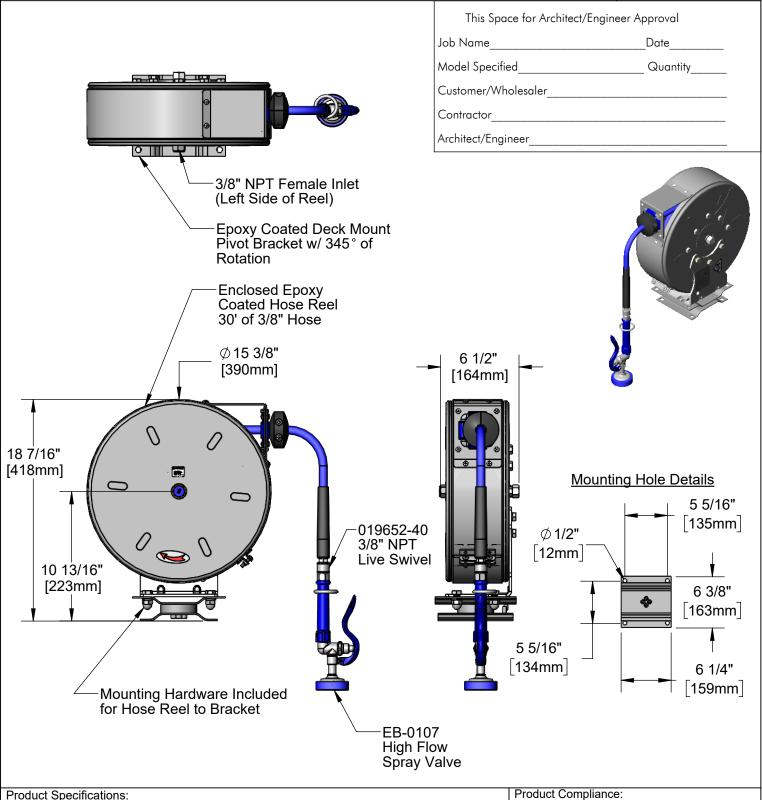
3/8" x 30' Enclosed Epoxy Coated Reel, High Flow Spray Valve & 345 Degree Epoxy Coated Pivot Deck Mount Bracket w/ Mounting Hardware for Hose Reel to Bracket
