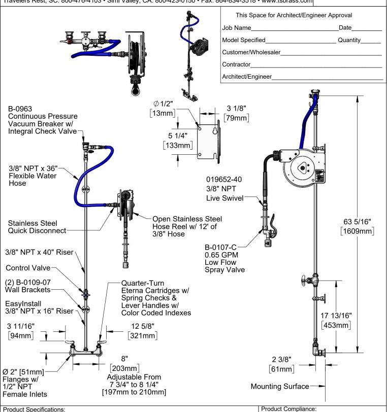
Open Stainless Steel Hose Reel w/ 12' of 3/8" Hose, 8" Wall Mount Faucet, Quarter-Turn Eterna w/ Spring Check, 0.65 GPM Low Flow Spray Valve w/ Swivel, Vacuum Breaker, 3/8" NPT Flexible Water Hose, Wall Brackets & Control Valve
