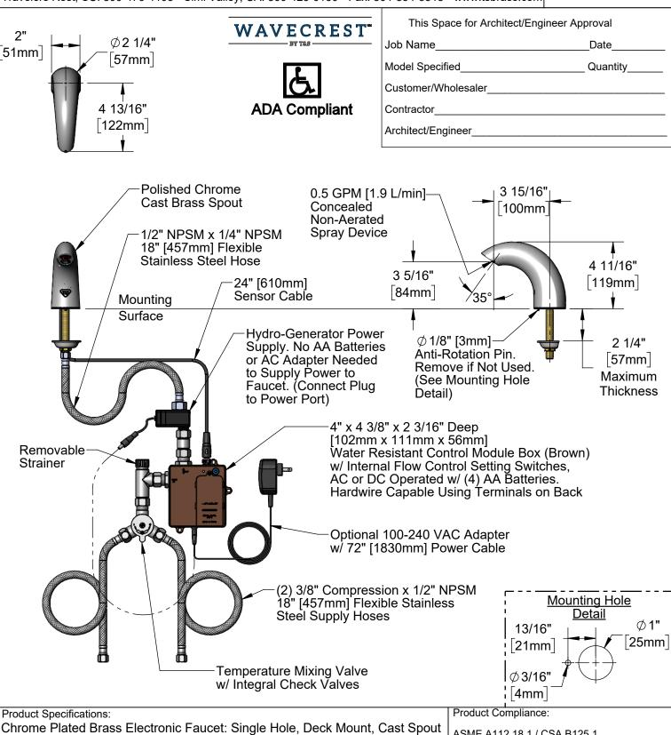
Integral Check Valves, Hydro-Generator & 18" Hot & Cold Supply Stop Flexible Connector Hoses
