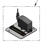
Flow Control Switches are Located Behind Battery Compartment Cover.
