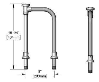
Pipe must be held rigid under sink with connection fittings,
