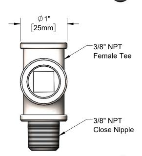
Note: 3/8" Hex L-Key Required to Remove Existing Swivel Piece (if Present on Pre-Rinse Unit) from EasyInstall Riser.
