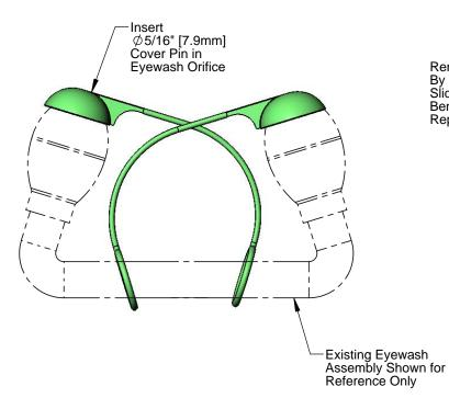
Remove SP11 Eyewash Head By Turning Counter Clockwise. Slide Ring End Over Eyewash Bend. Reinstall Eyewash Head. Repeat on Opposite Side.
