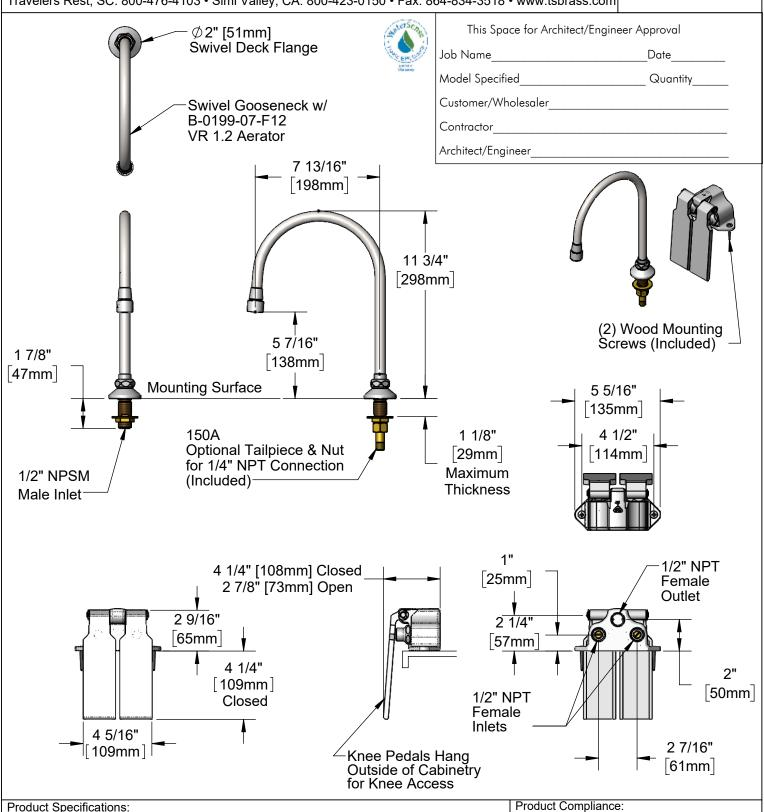
Ledge-Mounted Double Knee Pedal Valve w/ Deck Mount Dummy Rigid/Swivel Gooseneck & VR 1.2 GPM Aerator
