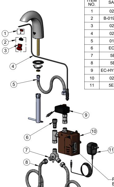
**ITEM** DESCRIPTION SALES NO. 020756-45 Curved Hidden Sensor w/ Screw B-0199-M21-V05 0.5 GPM Concealed Spray Device, M21.5 x 1 020674-45 M21.5 x 1 Red Cache Key 020754-45 WaveCrest Sensor Cable 016297-45 Inlet Hose, Faucet, 1/2" NPSM-F x 1/4" NPSM-F **EC-FILTER** Replacement Filter 5EF-0006 Temperature Mixing Valve 5EF-0005 Supply Hose, 9/16-24 Female x 1/2" NPSM **EC-HYDROGEN-LF** Low Flow Hydrogenerator WaveCrest Control Module w/ Filter Tee 020744-45 5EF-0002C AC Adapter - US Plug
