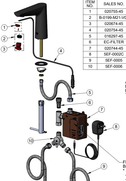
ITEM DESCRIPTION Straight Hidden Sensor w/ Screw B-0199-M21-V05 0.5 GPM Concealed Spray Device, M21.5 x 1 M21.5 x 1 Red Cache Key WaveCrest Sensor Cable Inlet Hose, Faucet, 1/2" NPSM-F x 1/4" NPSM-F Replacement Filter WaveCrest Control Module w/ Filter Tee AC Adapter - US Plug Supply Hose, 9/16-24 Female x 1/2" NPSM Temperature Mixing Valve
