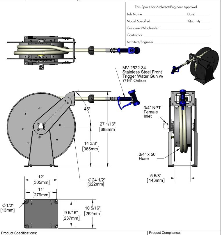
3/4" x 50' Open Coated Reel, Creamery Hose, Stainless Steel Front Trigger Water Gun, 7/16" Orifice & Double Arm Support
