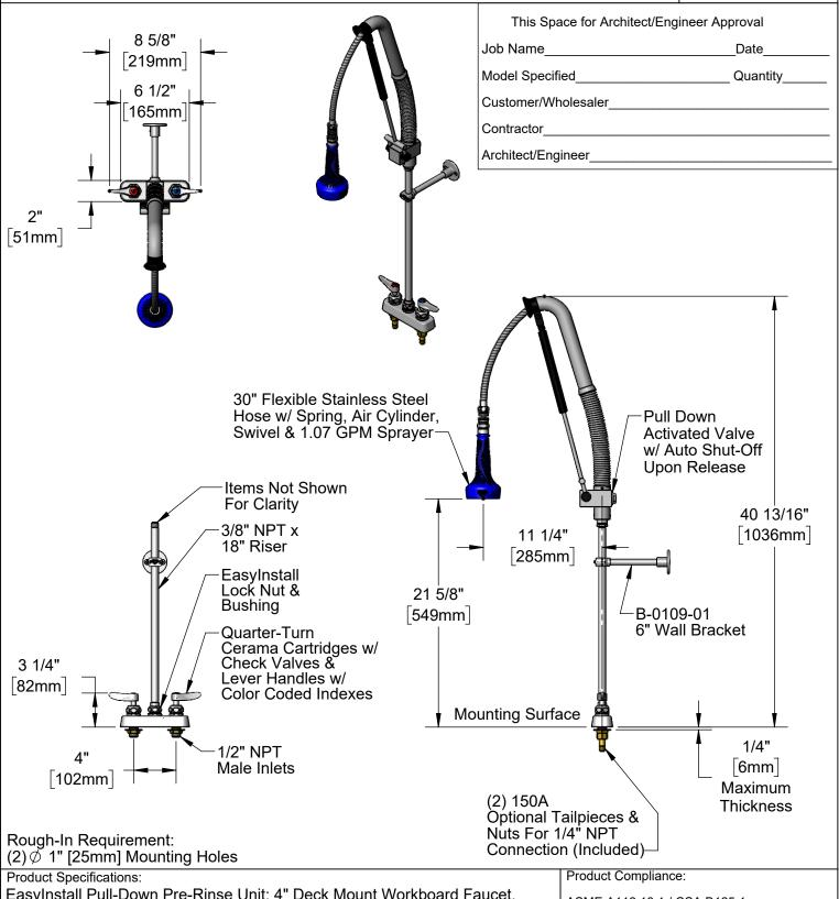
EasyInstall Pull-Down Pre-Rinse Unit: 4" Deck Mount Workboard Faucet, Quarter-Turn Cerama Cartridges w/ Check Valves, Lever Handles, 18" Riser, 30" Flexible Stainless Steel Hose, 1.07 GPM Sprayer w/ Ball-Joint Swivel, 6" Wall Bracket & 1/2" NPT Male Inlets
