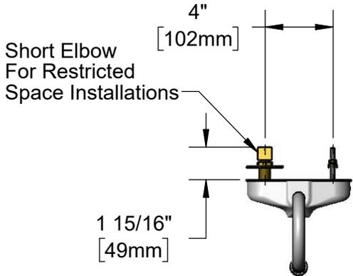
Rigid Gooseneck w/ 2.2 GPM [8.3 L/min] Vandal Resistant Aerator
