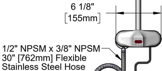
1/2" NPSM x 3/8" NPSM 30" [762mm] Flexible Stainless Steel Hose
