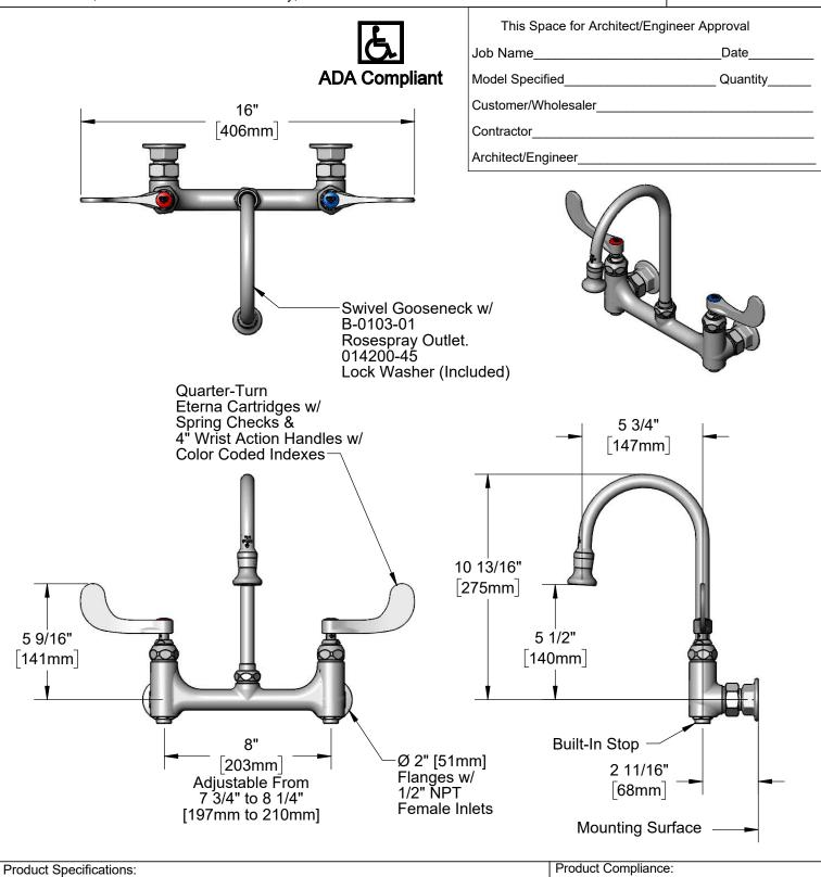
8" Wall Mount Mixing Faucet, Quarter-Turn Eterna Cartridges w/ Spring Checks, 4" Wrist Action Handles, 5 3/4" Swivel/Rigid Gooseneck w/ Rosespray Outlet, Built-In Stops & 1/2" NPT Female Inlets
