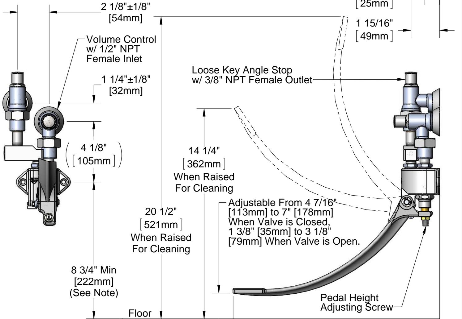
Note: All Pedal Position Dimensions are Based on Minimum Recommended Mounting Height of 8 3/4" [222mm] Above the Floor
