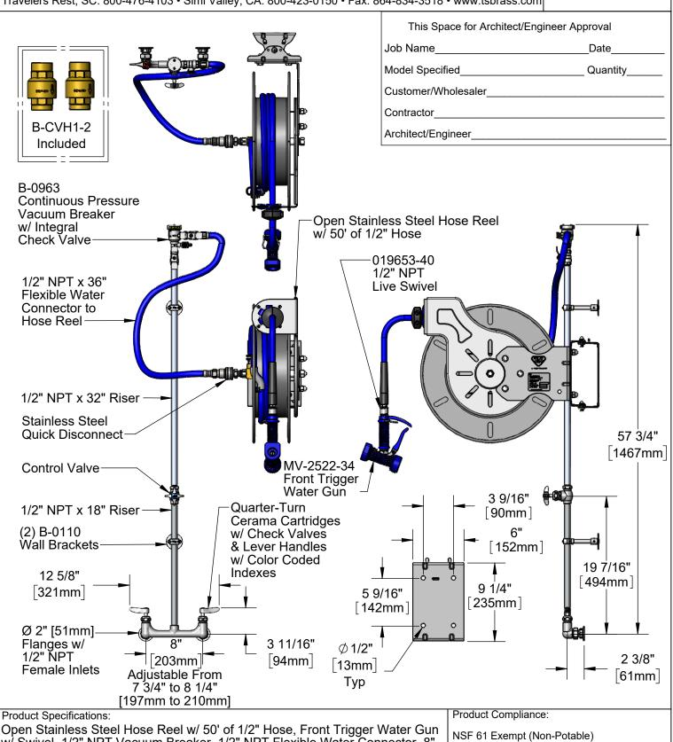
w/ Swivel, 1/2" NPT Vacuum Breaker, 1/2" NPT Flexible Water Connector, 8" Wall Mount Mixing Faucet, Control Valve, Horizontal Check Valves & Easylnstall Wall Swing Bracket
