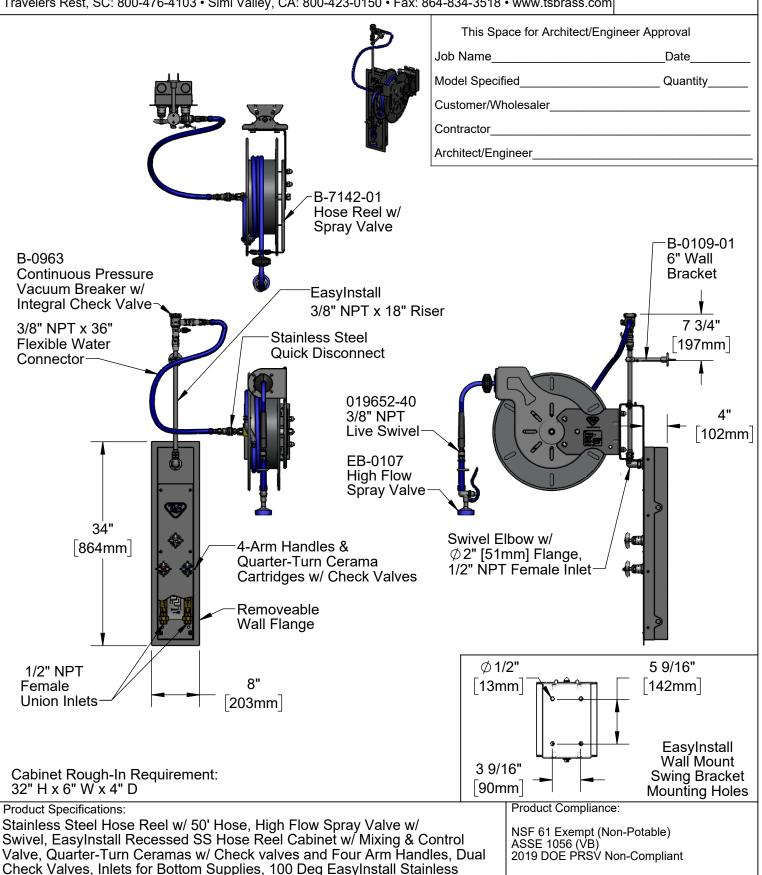
Steel Swing Bracket w/ Mounting Hardware & Hose Reel Connector Kit
