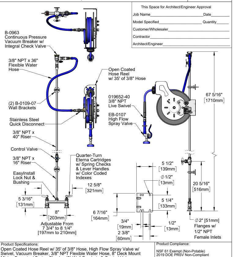
Mixing Faucet w/ Spring Checks, (2) Wall Brackets & Control Valve
