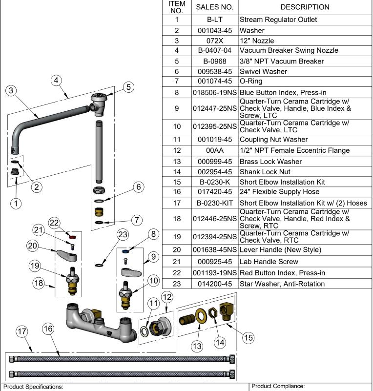
8" Wall Mount Mixing Faucet with Polished Chrome Plated Brass Body, Vacuum Breaker Swing Nozzle, Ceramic Cartridges with Check Valves, Lever Handles, 1/2" NPT Male Elbow Installation Kit with (2) 24" Flexible Stainless Steel Hoses
