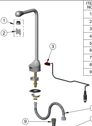
**ITEM** DESCRIPTION SALES NO. NO. VR 1.5 GPM Laminar Flow Device, 13/16-27 UN B-0199-08-LF15 Male w/ Key 2 Vandal Resistant Key 015425-45 019174-45 Sensor Cable Assembly 4 016297-45 Inlet Hose, Faucet, 1/2" NPSM-F x 1/4" NPSM-F ChekPoint Control Module w/ Filter Tee 019944-45 AC Adapter - US Plug 5EF-0002C Supply Hose, 9/16-24 Female x 1/2" NPSM 5EF-0005 002534-25 Close Nipple, 1/2" NPT **EC-FILTER** Replacement Filter
